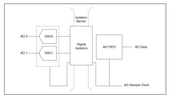
Figure 5-1. NI 6232/6233 Analog Output Circuitry
